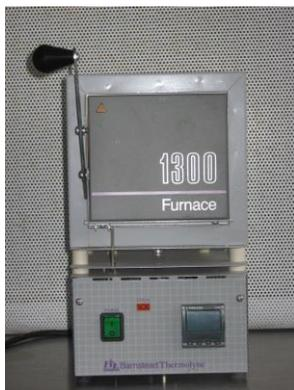
Figura 15. Mufla, Furnace 1300 Barnstead Thermolyne
